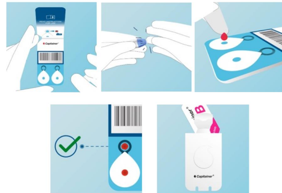
Figure 1. Capitainer®B is a next-generation quantitative dried blood spot (qDBS) microsampling card that collects an exact volume of 10 \mu\text{L} of capillary blood. The images depict the five simple steps in the self-sampling procedure. 1. Open and unfold the Capitainer®B card, 2. Prick the finger with the attached lancet, 3. Place a hanging drop of blood per microfluidic channel on the card, 4. Check that the test was successful using the inbuilt visual indicator, 5. Send the card by post to the laboratory in a prepaid envelope.
